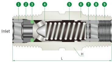
\* 701 Series is without Adjusting screw and locking screw
